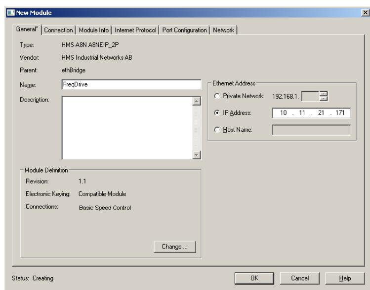
4. Enter a Module Definition e.g. Basic Speed Control, then press OK.
